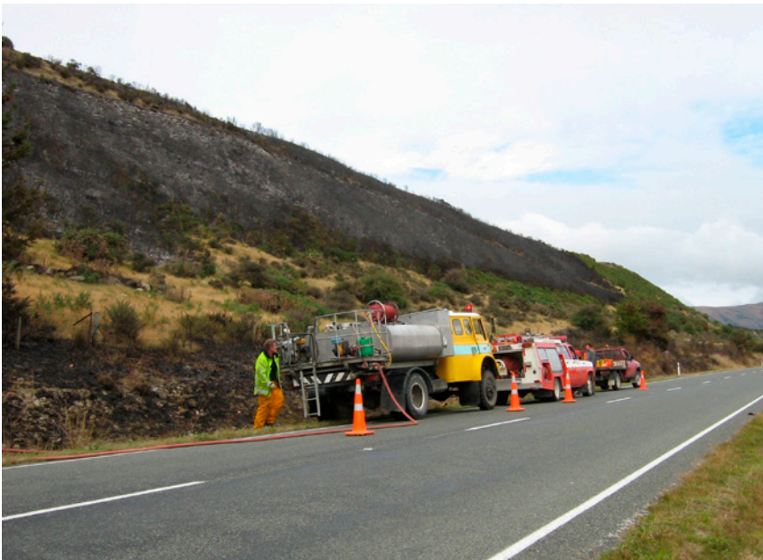
Figure 3.7 Parking on side of road ensures other road users see you
