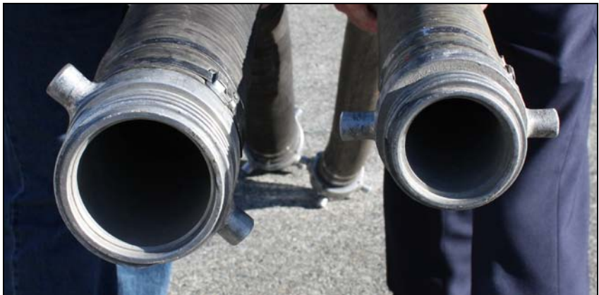
Figure 4.8 – 75 and 100 mm standard hose couplings
