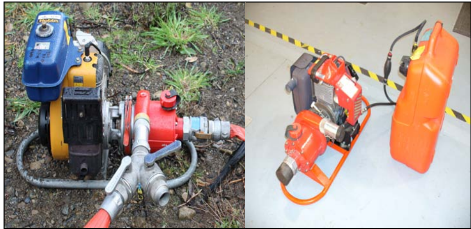
Figure 1.1 – Wajax pumps – left to right: MK V Robin engine; MK III Wick engine
