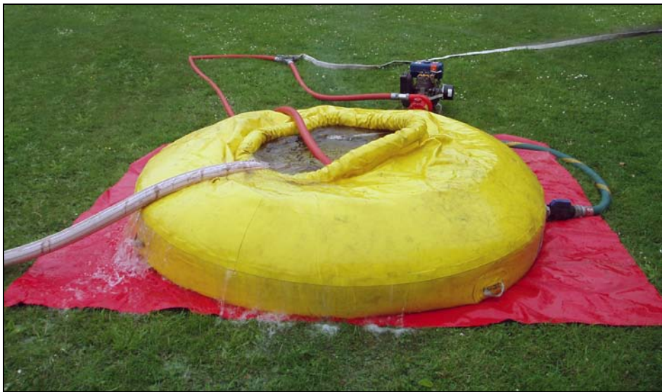
Figure 4.12 – Portable dam used as part of an open relay
