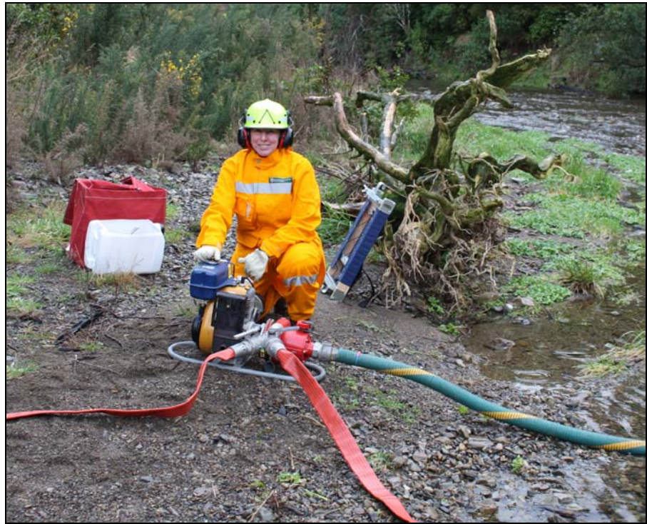
Figure 4.1 – A clear, level pump position and a pump operator wearing personal protection equipment (PPE).
