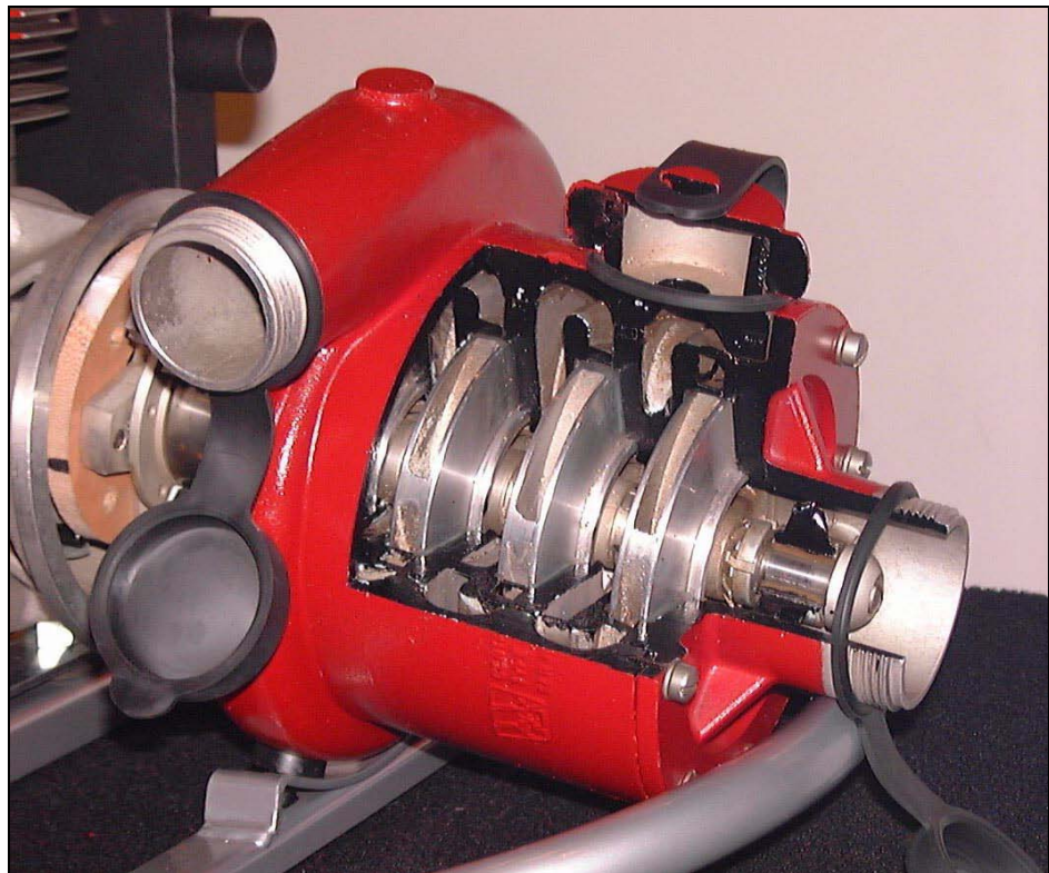
Figure 1.2 – Cutaway Wajax pump showing the arrangement of the impellers and distributors
