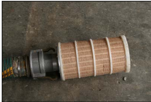
Figure 4.3 –75 mm camlock coupling with strainer
