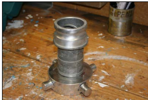
Figure 4.4 –75 mm camlock to 100 mm round thread adaptor for pump inlet
