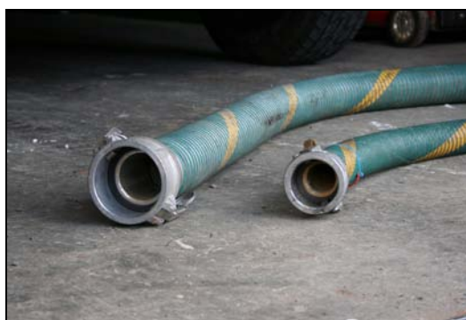
Figure 4.2 – 75 mm and 50 mm camlock with wire bound composite suction hose
