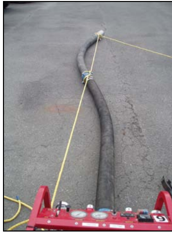
Figure 4.9 –Tying off suction hose
